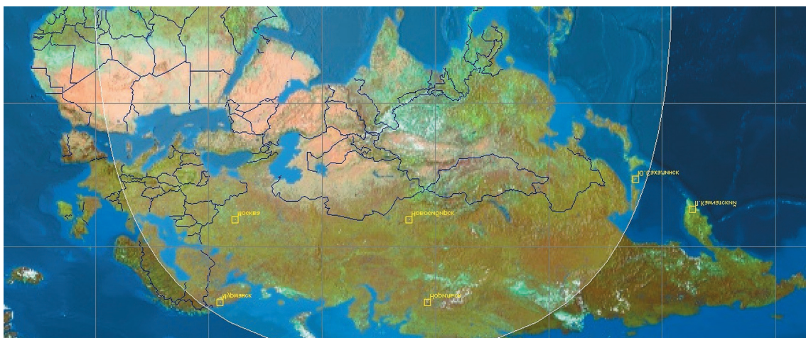
Fig. 3. Radio visibility zone during GEO SC operation.
