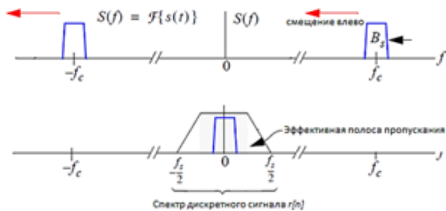
Fig. 3. The transmission of a signal into the zero frequency. (Shift to the left / Effective bandpass / discrete signal spectrum)
