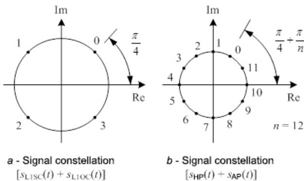
Fig. 2. Phase diagrams of GLONASS signals being consolidated
