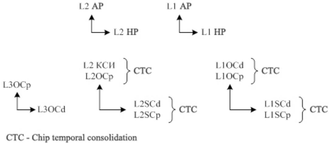
Fig. 1. Vector diagrams of GLONASS navigation signals
