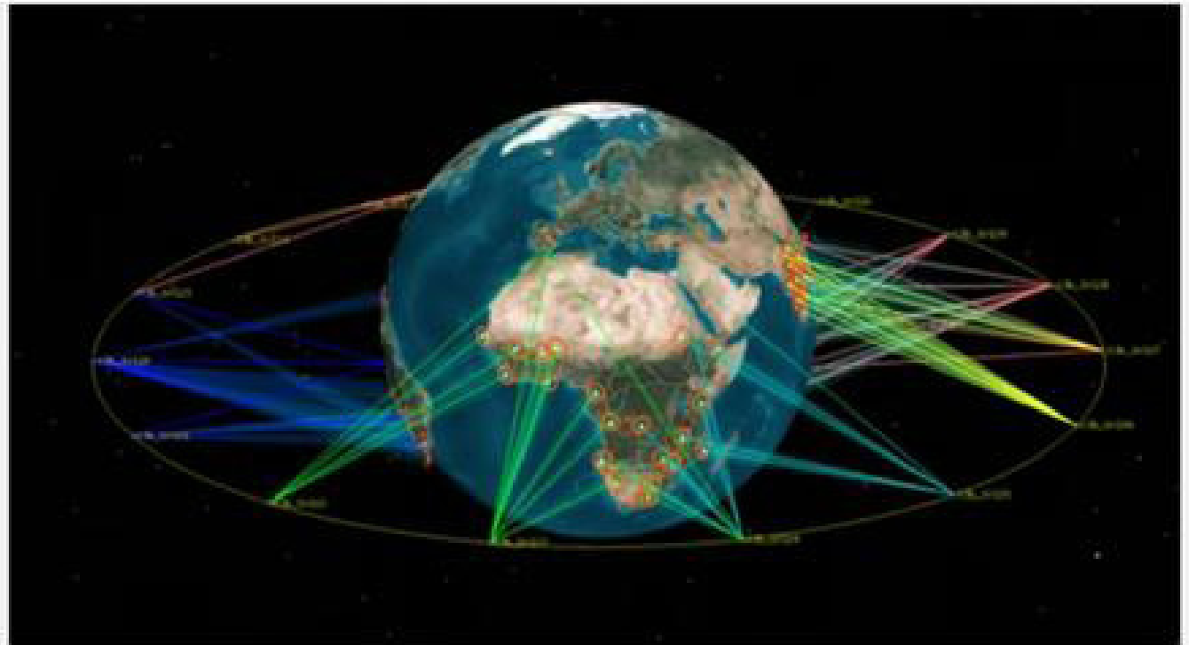
Fig. 1 Orbital formation of the O3b system: 16 satellites in a circular equatorial orbit with H = 8000 km.
