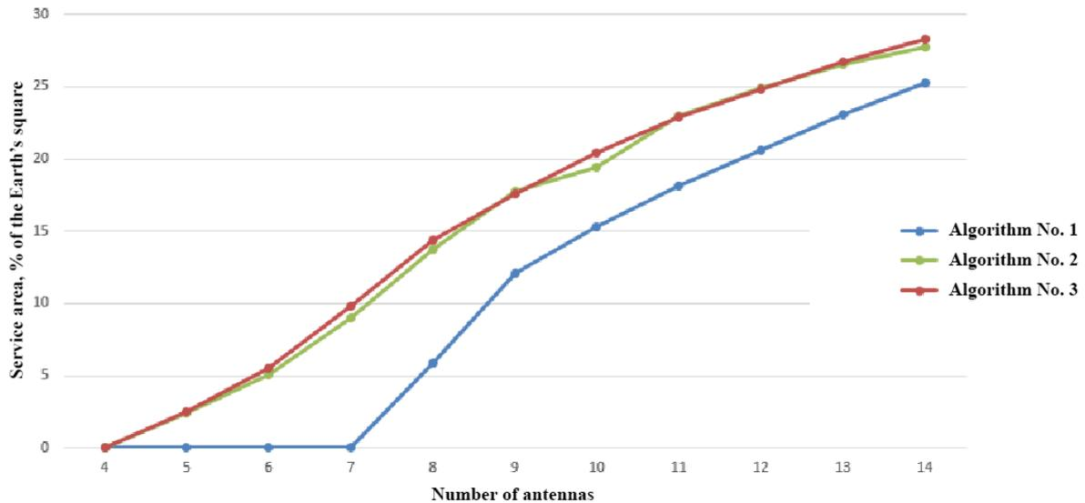
Fig. 5. Dependence of the size of the service area of the MEOLUT on the number of antennas with the assumption that all EPIRBs are movable
