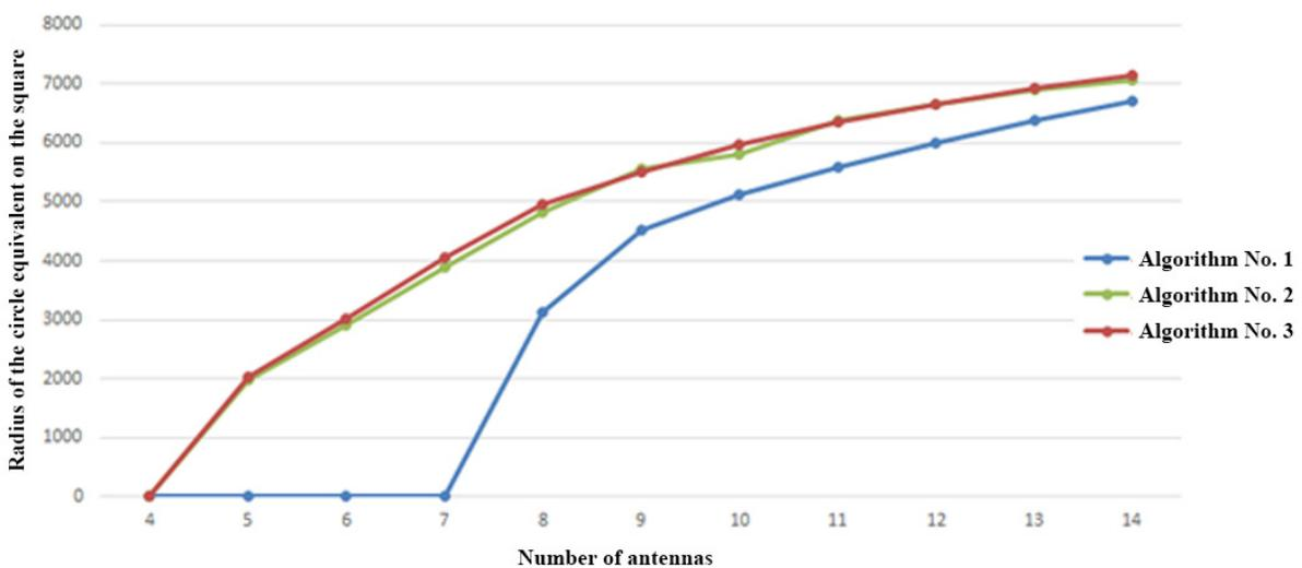
Fig. 6. Dependence of the radius of the circle equivalent as to the square of the service area of the MEOLUT on the number of antennas with the assumption that all EPIRBs are movable
