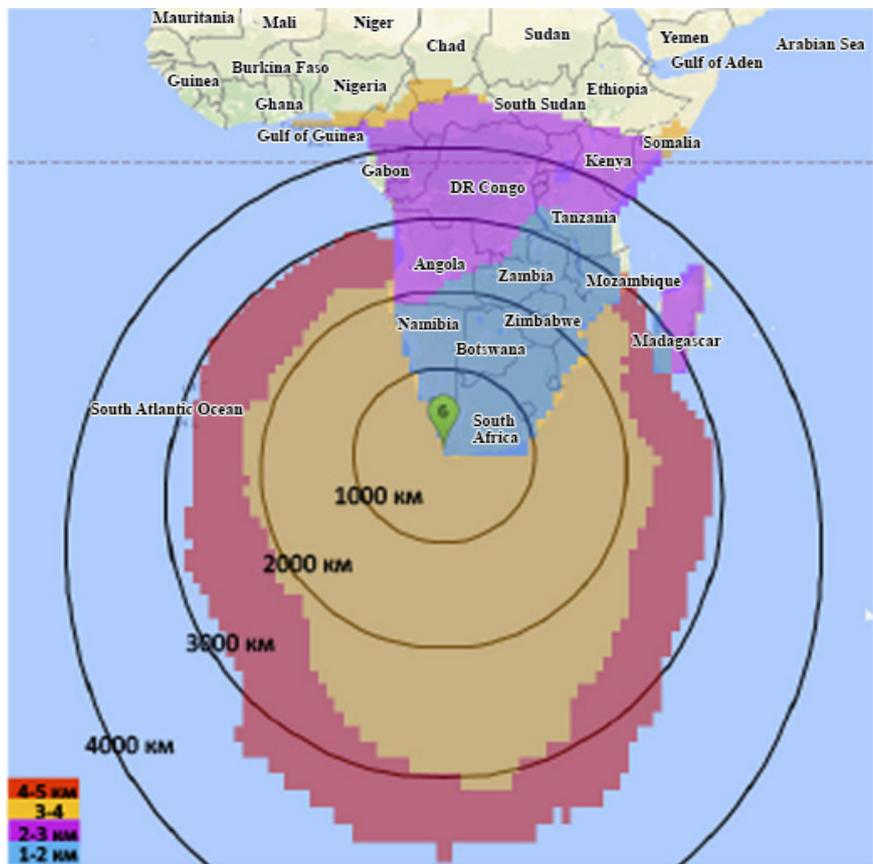
Fig. 4. Service area of the MEOLUT with six antennas in Cape Town
